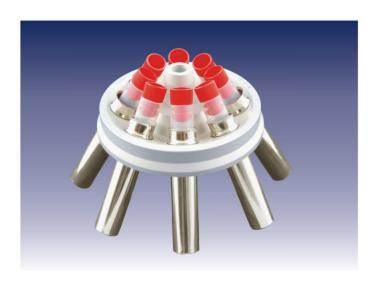
angle rotor 8x10 ml No 11145C with buckets 13080 max. radius R=8,3 cm angle 30° buckets with rubber pad No 13080 for tubes 10 ml (Ø 16x100 mm)
