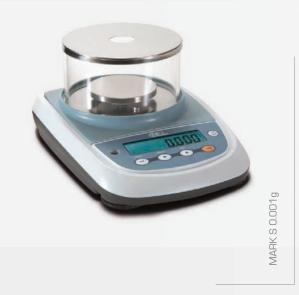
A fusion of design and quality, balances series S enclose all the experience of high-end models in a small footprint portable balance. Thanks to the sophisticated software and to a high-performance load cell, these balances are able to reach maximum capacity of 420 grams. The backlit LCD display, the RS232 interface and the many on-board software functions included make this balance a complete product at a very competitive price.
